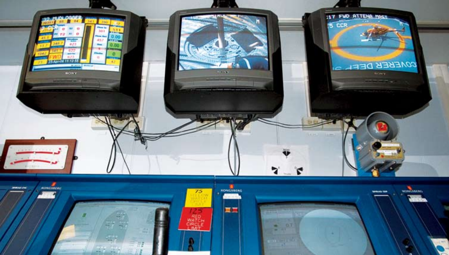
WEATHER EYE On the bridge, operators monitor (clockwise from upper left) drilling data, the moon pool, the chopper deck, and two depictions of the ship's position over the well.
